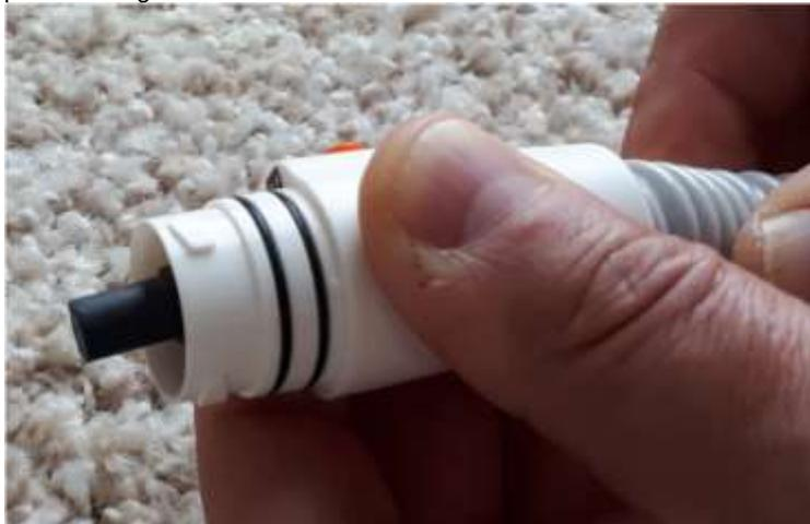
the connector can be pushed back out by squeezing the hose.
