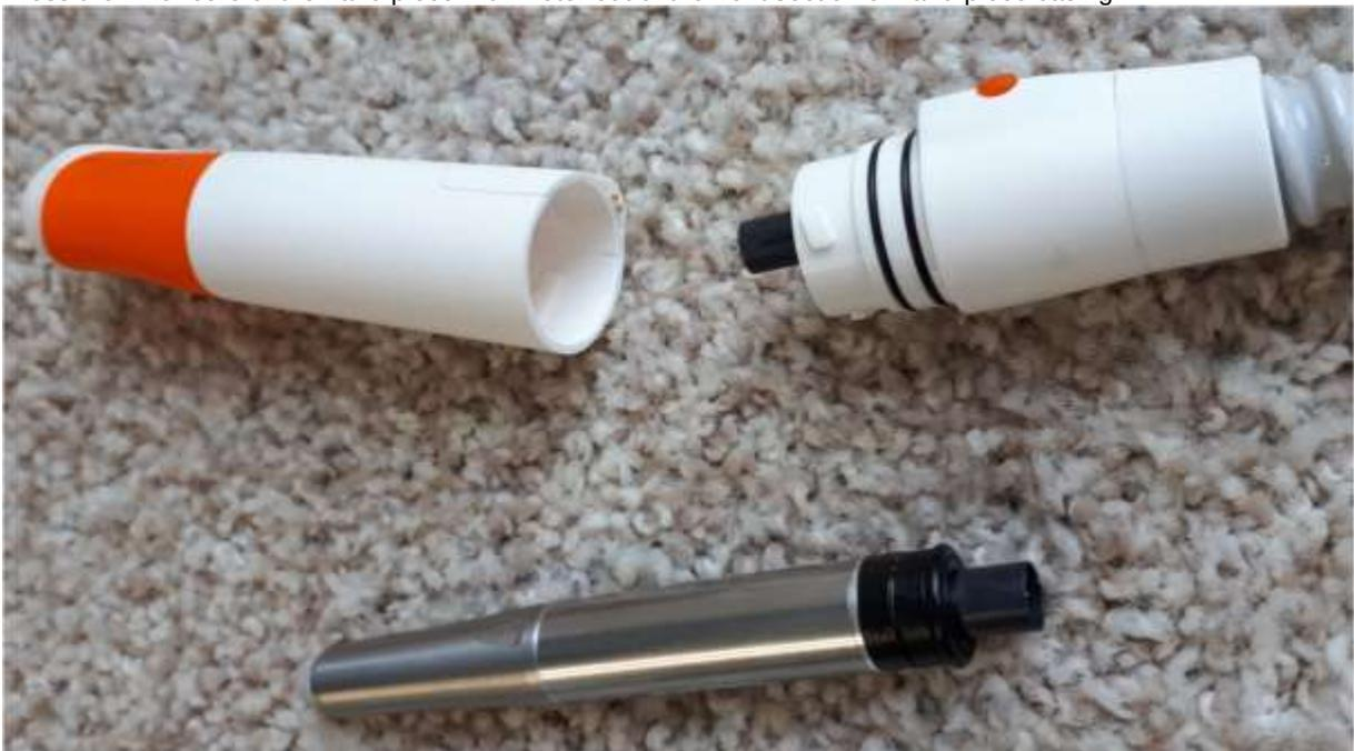
If necessary, disconnect the inner core of the hand piece with motor from the connector.
