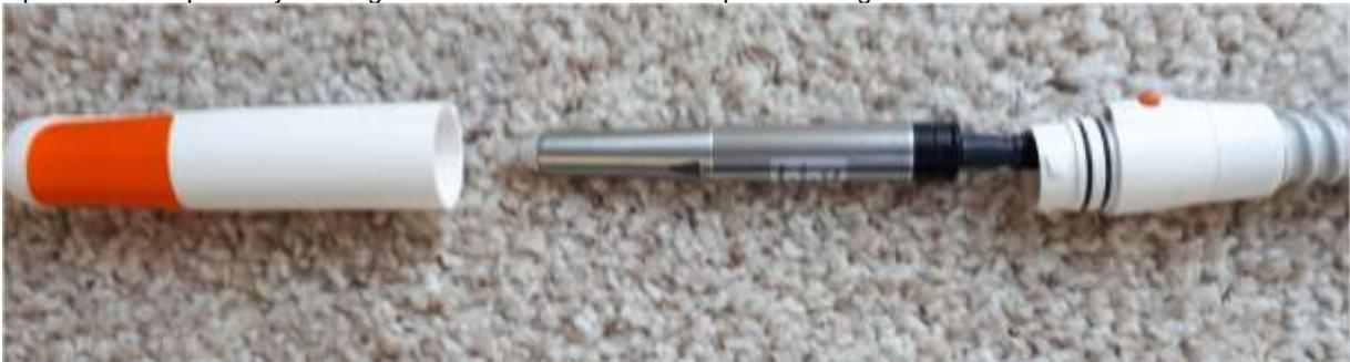
Press the inner core of the hand piece with motor out of the front section of hand piece casing.
